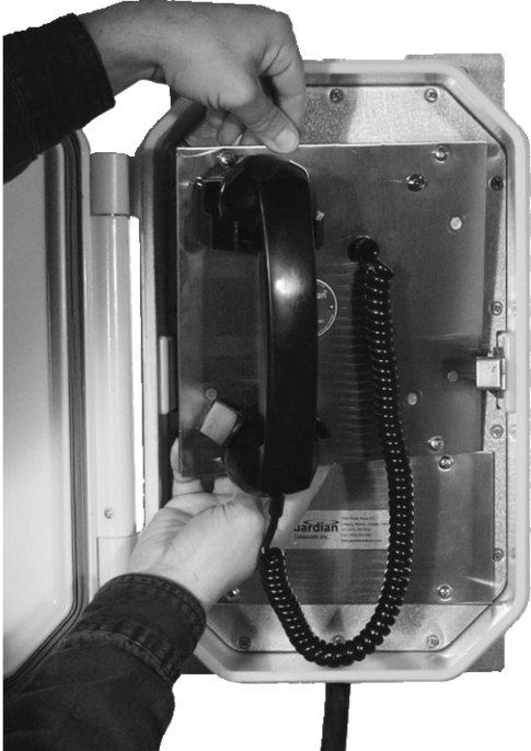
Figure 6 - PTR in Guardian Outdoor Housing
