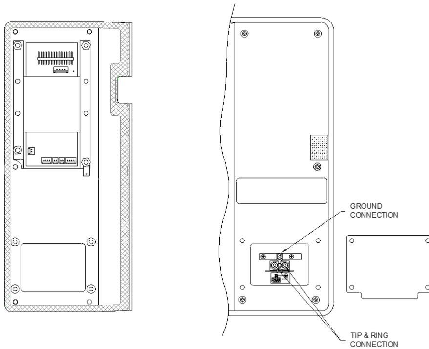
**Figure 5 - Tip & Ring Connection**
