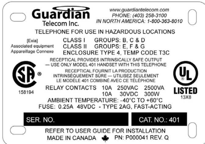
Figure 13 - I.D. and Compliance
